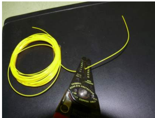
Figure 1.3: Stripping outer coating of optical fiber.
