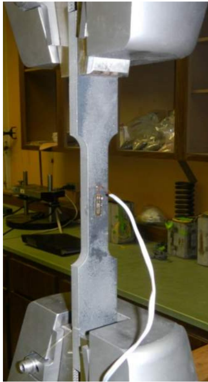
Figure 4.4. Test Setup for Strain Transfer of Surface Adhered FBG on Steel
