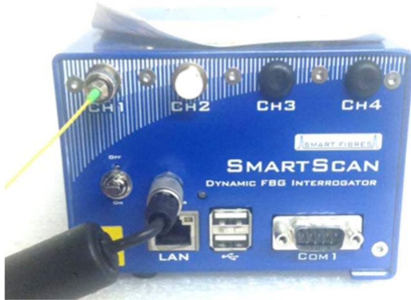
Figure 8: SmartScan Interrogator for Fiber Bragg Grating Sensors
