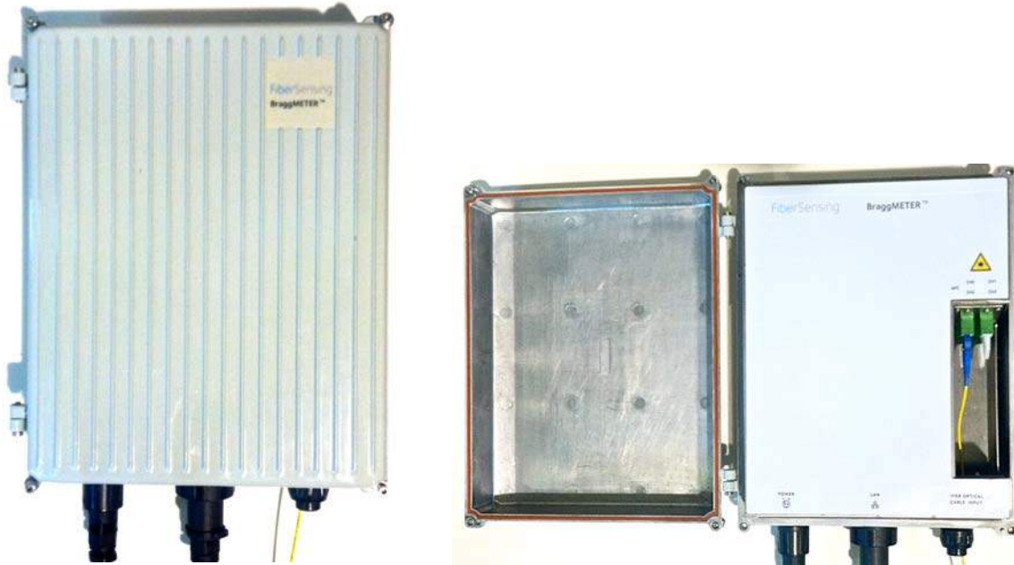
Figure 36: Exterior Top View (left) and Interior View with FBG Inputs (right) of Interrogator
