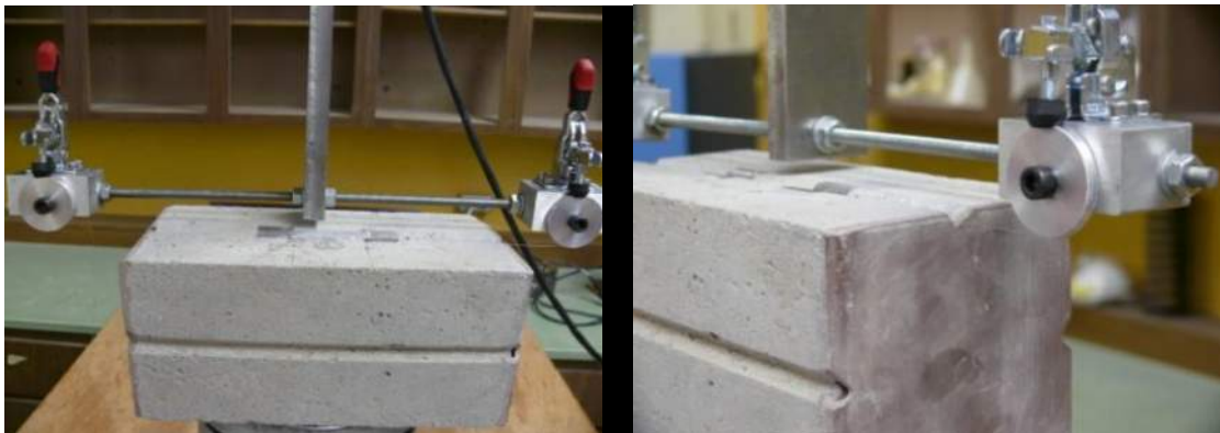
Figure 4-5: FBG notch embedment setup
