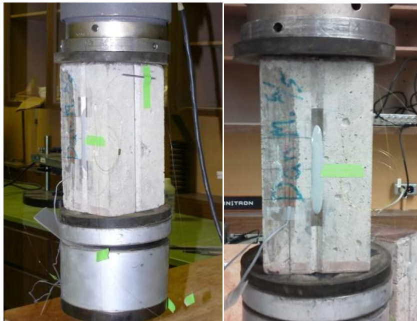
Figure B2: Axially loaded concrete prism test setup
