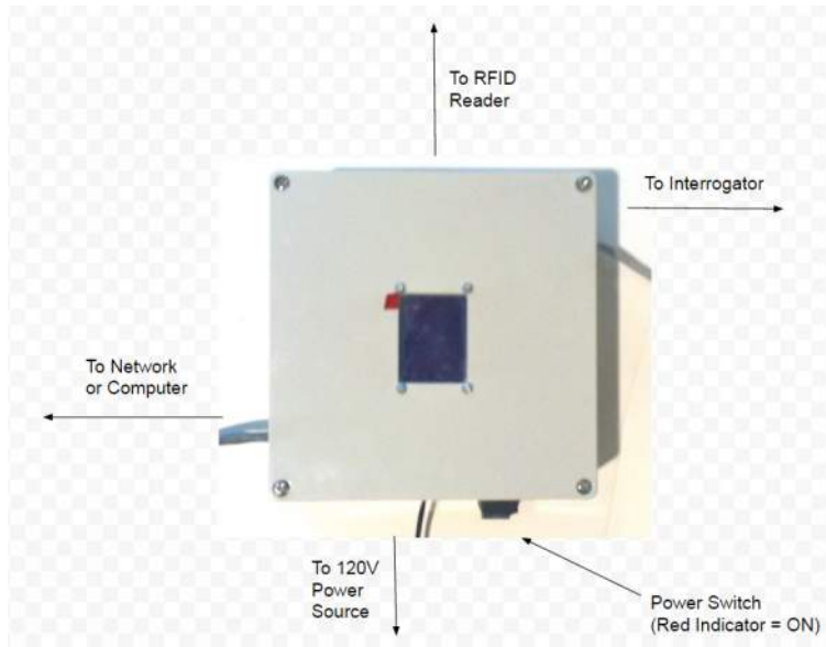
Figure 5.8: Diagram of appropriate connections to the data controller
