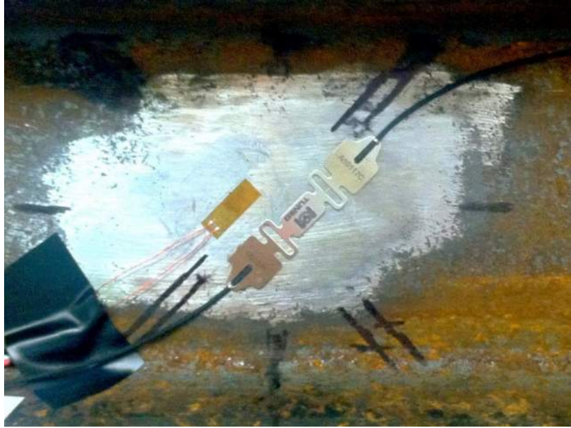
Figure 11: Traditional Foil Gage (left) and Micron Optics' os3120 Sensor (right)
