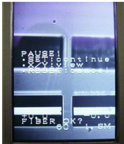
Figure 1.9: Well Prepared Fibers
