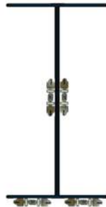
Figure 6.1 – Cross-Sectional View with FBG Sensors on the Web and Bottom Flange
