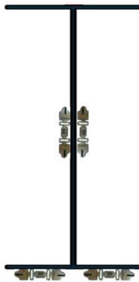
Figure 26: Cross-Sectional View with FBG Sensors on the Web and Bottom Flange
