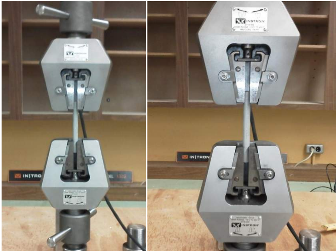
Figure B6: Epoxy stiffness test
