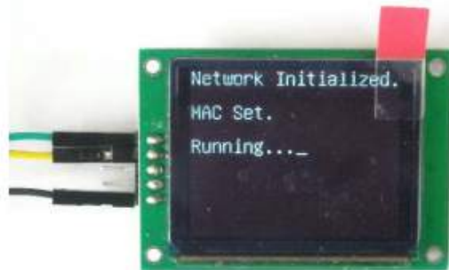
Figure 5.9: Data controller OLED Screen indicating a successful startup
