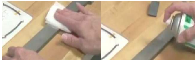
Figure 49: Step 2 - Surface Preparation
