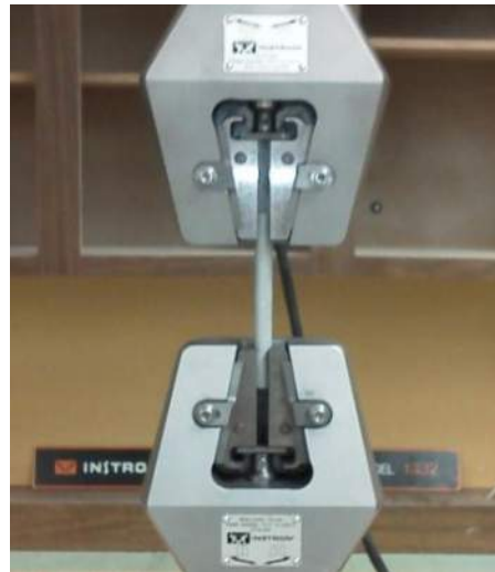
Figure 4-4: Epoxy stiffness test
