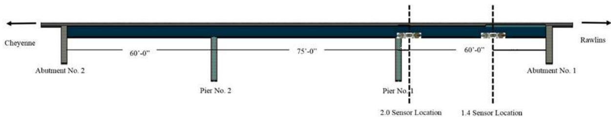
Figure 27: Elevation View with Critical Locations for Sensor Placements
