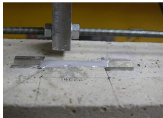
Figure 4-6: Epoxy bond length
