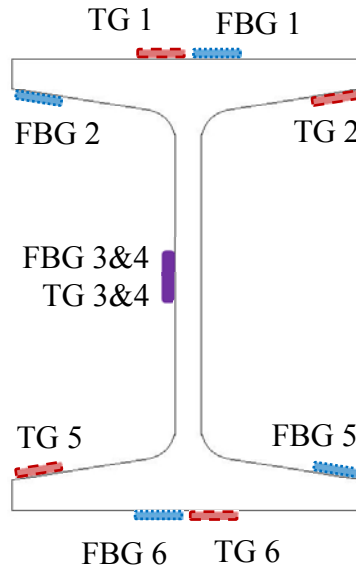
Figure 16: Cross-Section View with Sensor Placement
