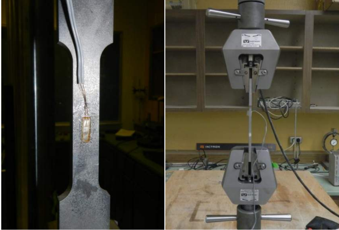
Figure B5: FBG gage factor calibration test
