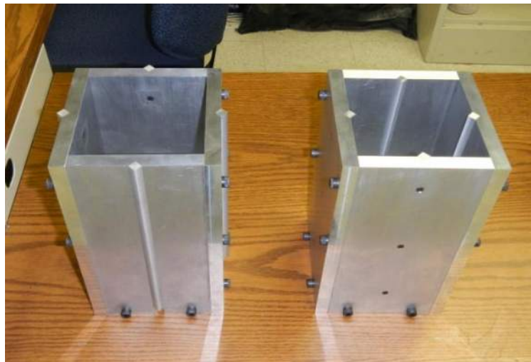
Figure 4-1: Concrete prism forms
