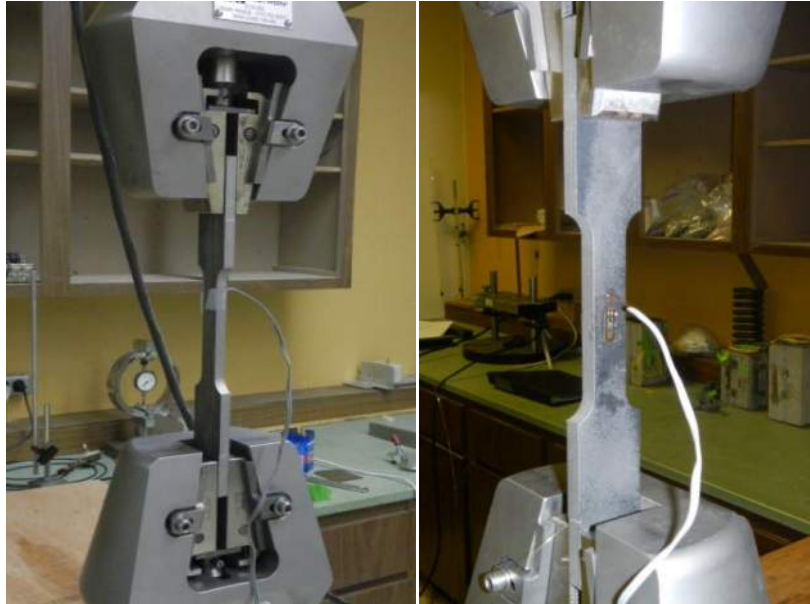
Figure 4-16: Steel dogbone gage factor calibration test
